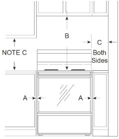
To reduce the risk of burns or fire when reaching over hot surface elements, cabinet storage space above the cooktop should be avoided. If cabinet storage space is to be provided above the cooktop, the risk can be reduced by installing a range hood that projects at least 5" beyond the front of the cabinets. Cabinets installed above the cooktop must be no deeper than 16".
