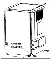
To prevent the range from tipping over due to improper use or overloading the open door, an antitip bracket (included in the package) must be installed properly by following instructions below. The anti-tip bracket can be fixed at either the left or right side of the appliance.
